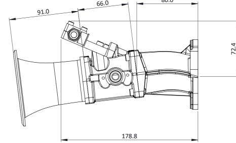
A KIT FOR THE HONDA K20 EP3 ENGINE WHICH CONTAINS A 7 DEG CURVED INLET MANIFOLD, FOUR 50mm THROTTLE BODIES WITH 51mm INLET, LEVERS, FUEL RAIL AND FOUR TAPERED AIRHORNS.
